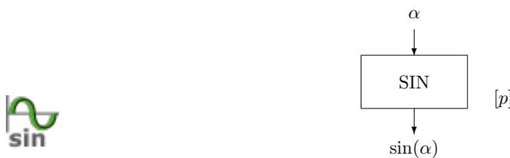
The SIN block requires exactly one input, namely an angle  $\alpha$ . It returns exactly one output, the sine of  $\alpha$ . The parameter  $[p]$  is written in square brackets, which means that the parameter  $p$  is optional, i. e. not necessarily required.
